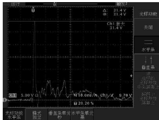
ESD Clamping Voltage Screenshot Positive 8 kV Contact per IEC61000-4-2
